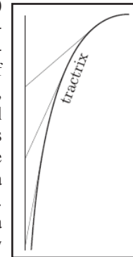
Figure 3. The tractrix, or the pursuit curve: all tangent segments have the same length.
