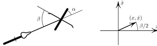
**Fig. 4.** The “handlebar angle”  $\beta$  evolves exactly as the doubled phase angle  $2 \arg(x + i\dot{x})$  of (4), provided that the front wheel’s path is generated by the potential  $p(t)$  via (5)–(6).
