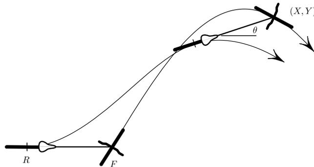
Fig. 1. An idealized bike. In this example  $F$  travels along an arc of a sine curve.
