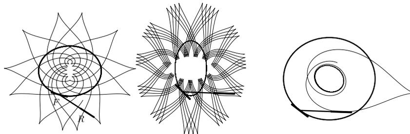
Fig. 3. The path traced out by the rear wheel as the front wheel repeatedly traverses a closed curve.
